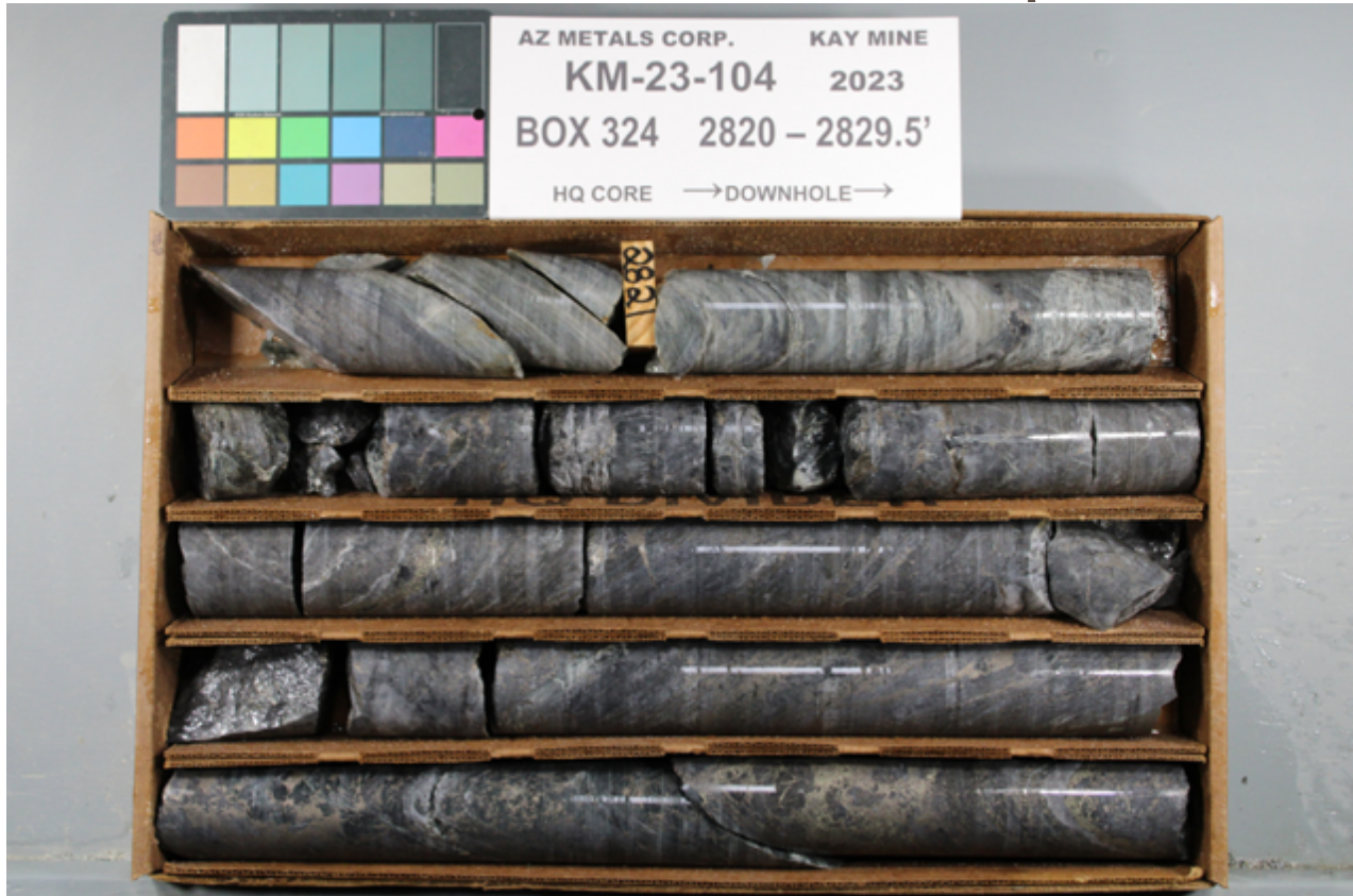
Figure 4. Core from hole KM-23-104 at the Western Target, displaying stringer to semi-massive sulfide mineralization hosted in a quartz crystal-rich volcanoclastic and breccia, with sulphide mineralization including pyrite, pyrrhotite, sphalerite, and chalcopyrite.
