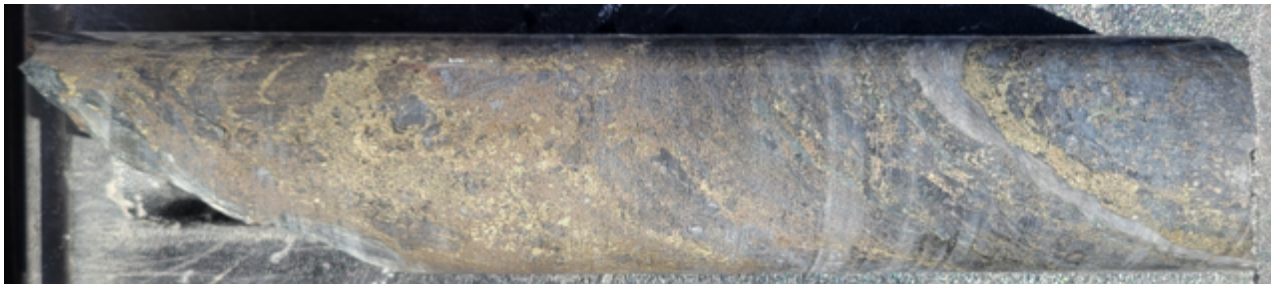
Figure 5. Core from hole KM-23-104 (at 2,829' downhole) at the Western Target, displaying stringer to semi-massive sulfide mineralization including stringers of sphalerite and flecks of chalcopyrite.
