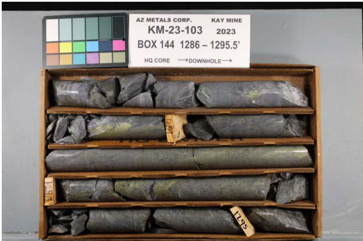
Figure 4. Core from hole KM-23-103 between 392.2 m and 395.1 m downhole, which includes an interval of 1.5 m grading 7.6% copper, 1.8 g/t gold, 2.6% zinc, and 26 g/t silver. This is part of a broader interval of 10.5 m grading 6.2% CuEq. See Table 1 for constituent elements, grades, metals prices and recovery assumptions used for CuEq % calculations. Analyzed metal equivalent calculations are reported for illustrative purposes only.
