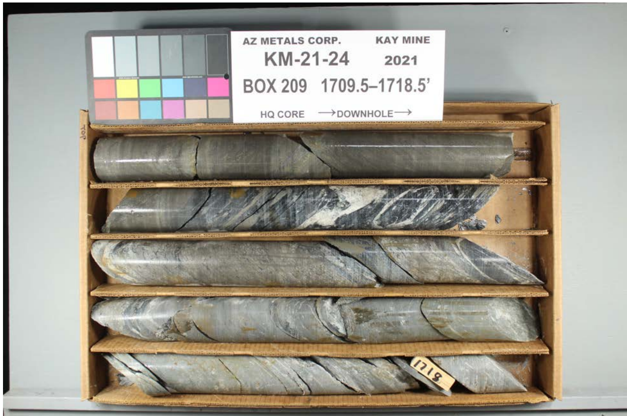
Figure 2. Hole KM-21-24 displaying interval from 520.9 m to 521.7 m downhole, containing 0.8 m of 33.4 g/t AuEq (comprised of 16.5 g/t gold, 574 g/t silver, 1.75% copper, 1.22% lead, and 9.55% zinc). See Table 2 for constituent elements and grades of AuEq g/t.
