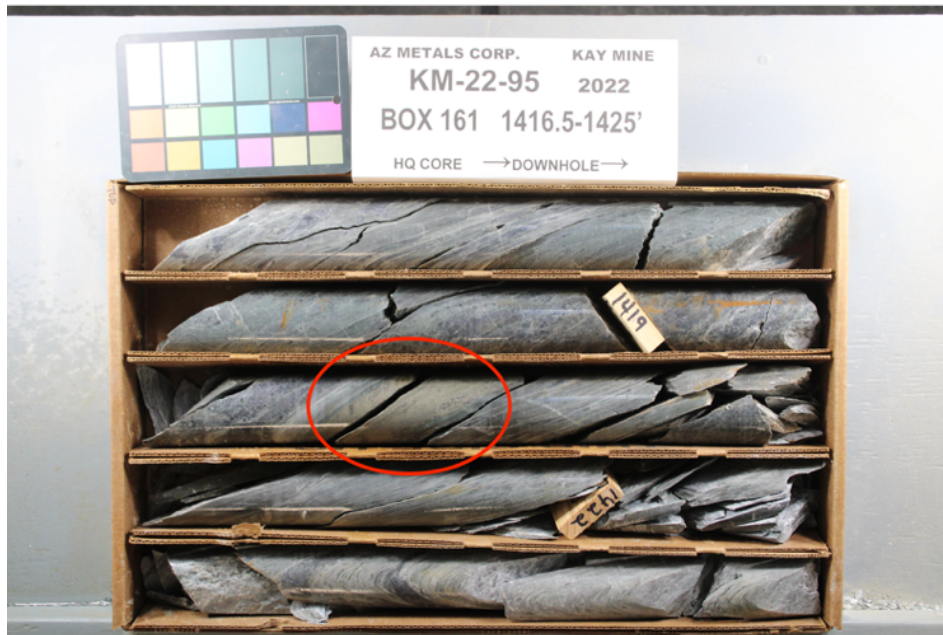
Figure 3. Core from hole KM-22-95 displaying a layer, likely a clast (circled in red) of sphalerite (zinc sulphide) and chalcopyrite (copper sulphide) massive sulphide at a depth of 433 m. This clast, part of the interval of 2.7 m grading 0.5% CuEq (from 432.8m to 435.5m) is indicative of proximity to primary massive sulphide mineralization.
