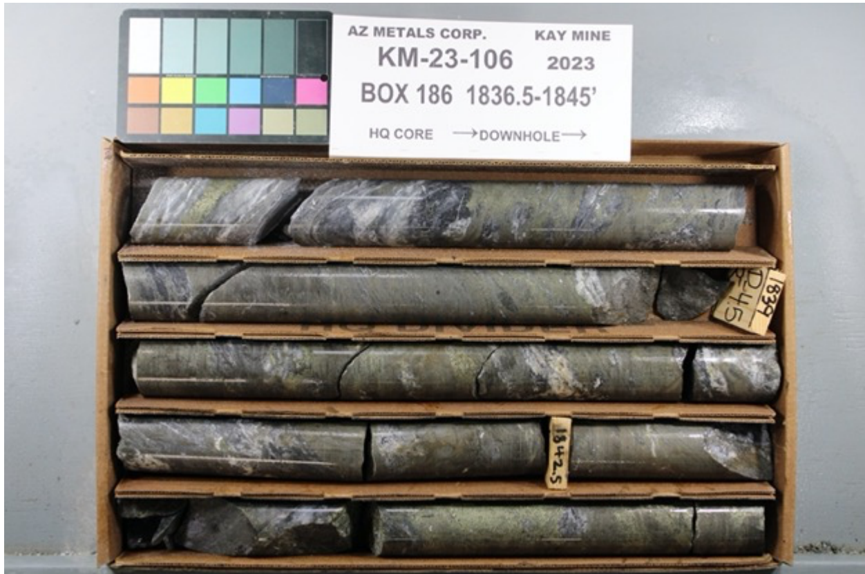
Figure 4. Core from hole KM-23-106 between 559.8 m and 562.4 m downhole, which is part of a broader interval of 10.4 m grading 5.1% copper, 3.1 g/t gold, 0.5 % zinc, and 23 g/t silver. See Table 1 for constituent elements, grades, metals prices and recovery assumptions used for CuEq % calculations. Analyzed metal equivalent calculations are reported for illustrative purposes only.
