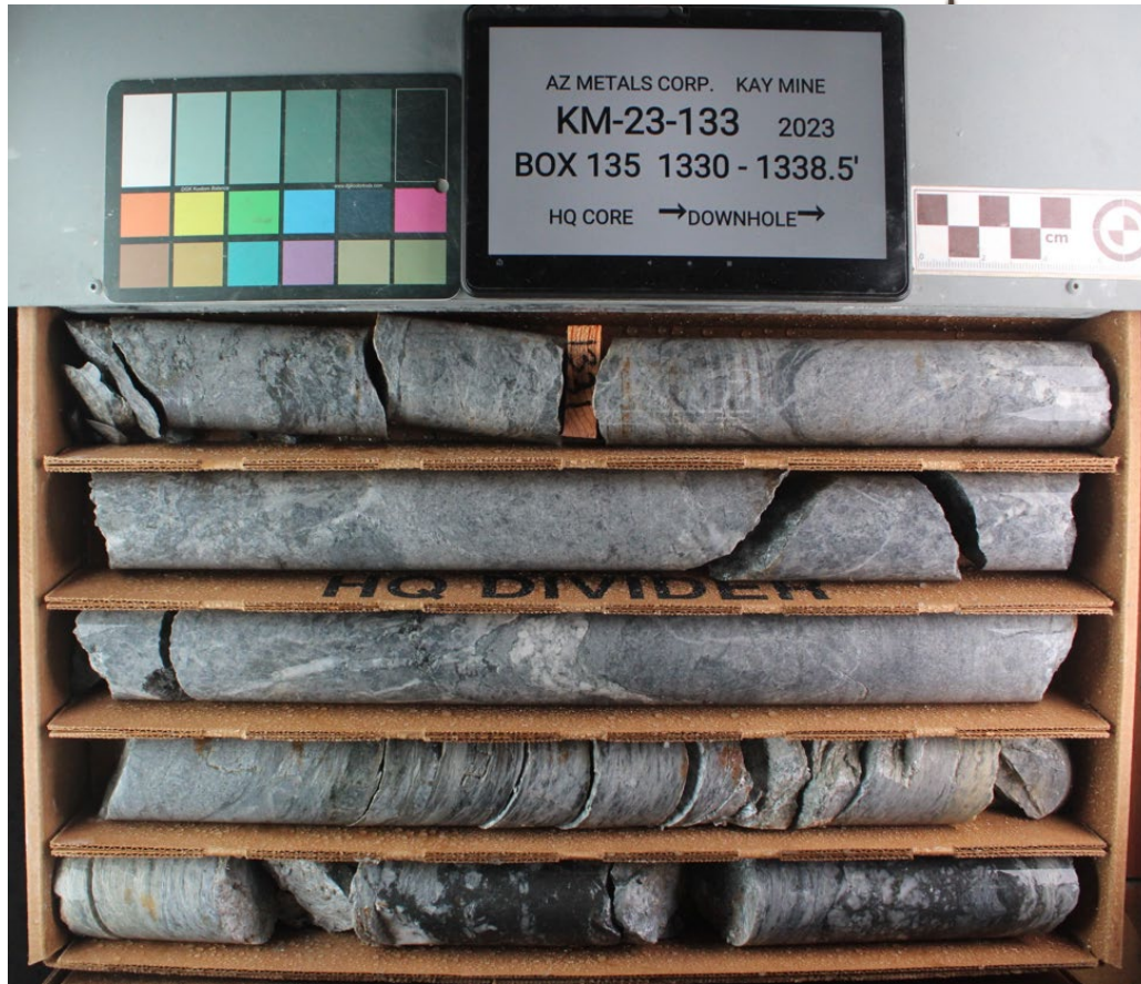
Figure 3. Drill core from Hole KM-23-133, showing the 0.5 m interval 407.5 m to 408 m which intersected 28.7 g/t gold, 7.1% copper, 0.99% zinc, and 564 g/t silver (for an equivalent grade after assumed recoveries of 36.8 g/t AuEq).
